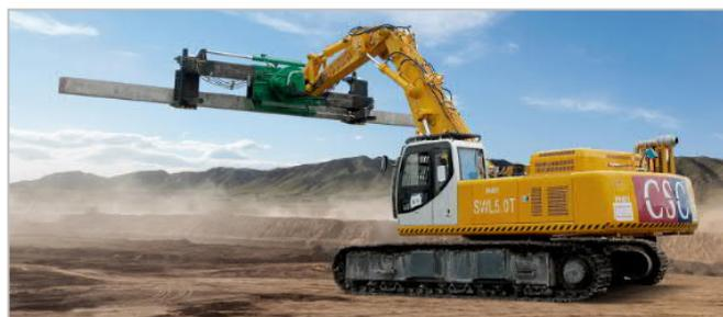
With the RC Pile Handler, the pile sections are lifted by a pair of forks and secured with a pair of clamps before being transferred efficiently and safely to the desired location within about two-thirds of the time.
