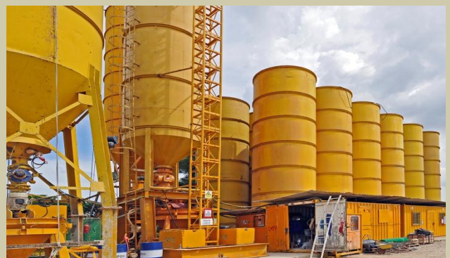
12 Silos, 3 ATM50 Mixers and 3 Agitator Tanks are set-up to store and supply Cement - Bentonite Slurry.
